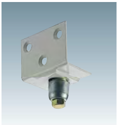
Retrofit Guide Roller #3 GRL •Common with #3 •Applicable door thickness: 30~50mm •With 3 pcs of Nominal dia: 5 x 25 countersunk tapping screw. •Make sure to fasten the roller tightly as it is temporary fixed state when shipped.
