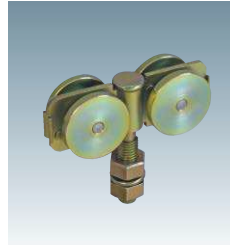
4-Wheel with Bearing [Flexible Type] #3 4WH-BN Load Weight: Up to 150kg/hanging 2 pcs
