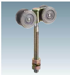
Wheel With Long Bolt #3 4WH-2LB Load Weight: Up to 150kg/hanging 2 pcs
